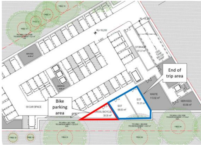
Figure 41 Bicycle parking and end of trip facilities
